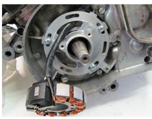
Unscrew the new stator coil from the base plate and lift it a little away from it so that you can access the mounting holes. Take care not to damage the paint insulation of the coil.
