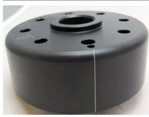
Take a look at the new rotor. You will find on its circumference a small pressed in line. That is an ignition marking. It is durable, but not well visible, so better highlighten it with some marker pen.
