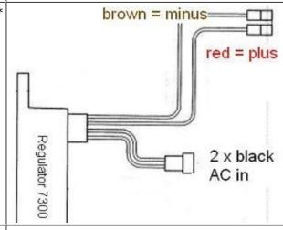
The new regulator/rectifier has 4 wires
