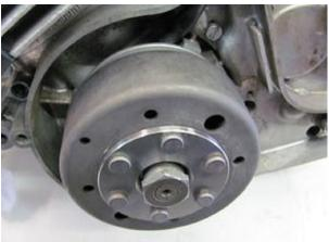
In this position fasten the rotor carefully by the supplied nut. Put the three provided washers under the nut (see pictur below).
