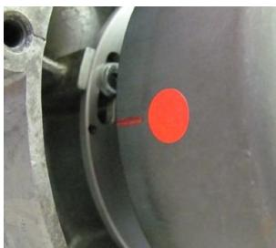
Take the spark plug out to ease turning of the crank and bring the piston into ignition position (put the rotor loosely onto the crank shaft and using it as a turning knob). Please consult your manual of the bike.
