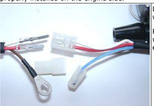
Look for the ignition coil with its female plug and the two wires (red and white).
