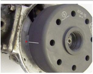
Carefully remove the rotor again from the crank (best using the puller tool for this) and reset it in such a way that the marking on the rotor aligns with the (transferred) marking of the stator. If there is any change in the crank's (ignition) position, you have to start again.
