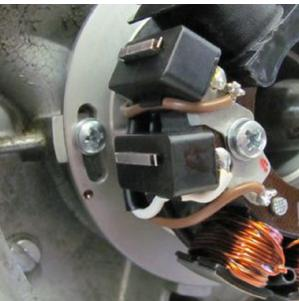
Have a look at the new stator unit. You will find at the adapter plate, near the black coils, a small red dot, this is an ignition marking.
